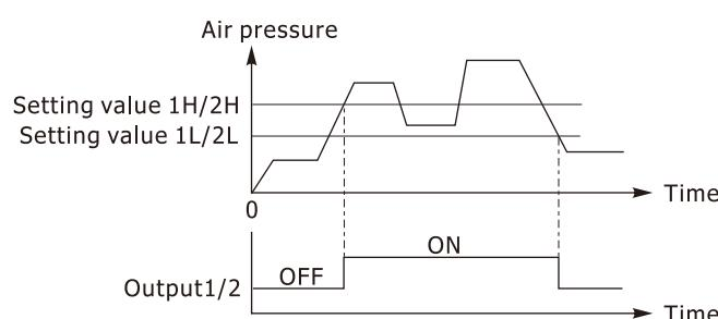
3. Window comparator mode: Set the pressure value H/L. When the pressure is greater than the H value or less than the L value, the output is OFF; when the air pressure is greater than the L value and less than the H value, the output is ON.
