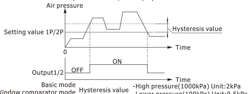
2. Hysteresis mode: Set the pressure value 1H/2H/1L/2L. When the applied pressure value is greater than 1H/2H, the display will ON. When the applied pressure is less than 1L/2L, the display will OFF.
